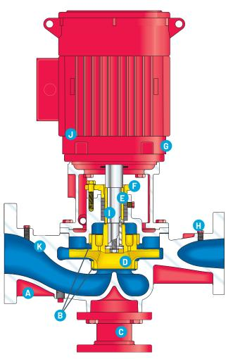
NOTE: Front case wearing rings are standard on all size pumps. Rear case rings are standard on all sizes except the 2x2x9C. The 2x2x9C does not require a wear ring.
